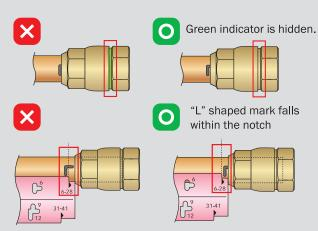
If the "T" or "L" shaped mark falls outside the notch in the marking gauge, cut off the joint, replace it with a new joint, and carry out construction again.
